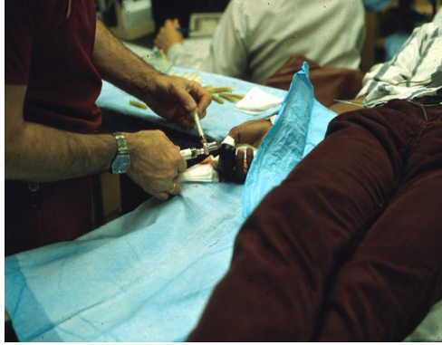
Fig. 4.1. In-vivo calibration of a pulse oximeter sensor conducted on a volunteer.
